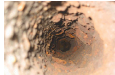
Internal view of 4» (DN 100) pipe due to corrosion
