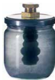
The magnet rod from the Zeparo can hold 143 g iron balls
