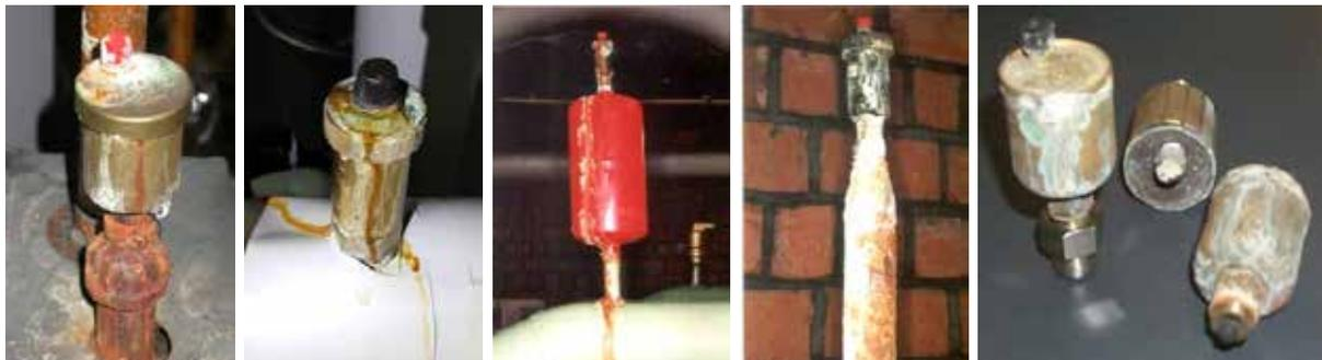
Example of poor-quality air vents, which soon begin to leak due to their faulty construction
