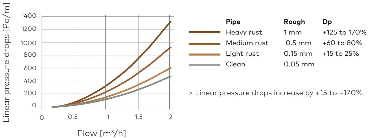
(\*) If a pipe pressure drop represents 50% of the total pressure drop of the system, a 70% increase in pipe pressure drop will have a direct 35% impact on electrical pipe consumption to achieve the same flow. (\*\*) Source: Result published by Utah State University, Pr Rahmaye.
