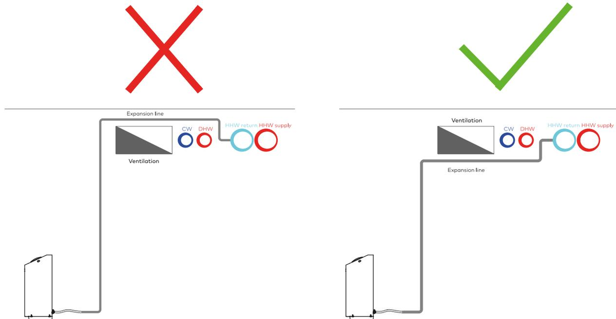
The connection DNe should be sized in accordance with the diameter required for the vacuum degasser and should contain flexible hoses to have a direct connection to the TecBox without tension.
