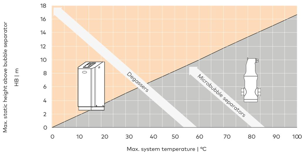
Microbubble separators are fully functional only below the line. Degassers that are capable of removing dissolved gases in addition to possible free gas bubbles are the solution when microbubble separators reach their physical limit.
