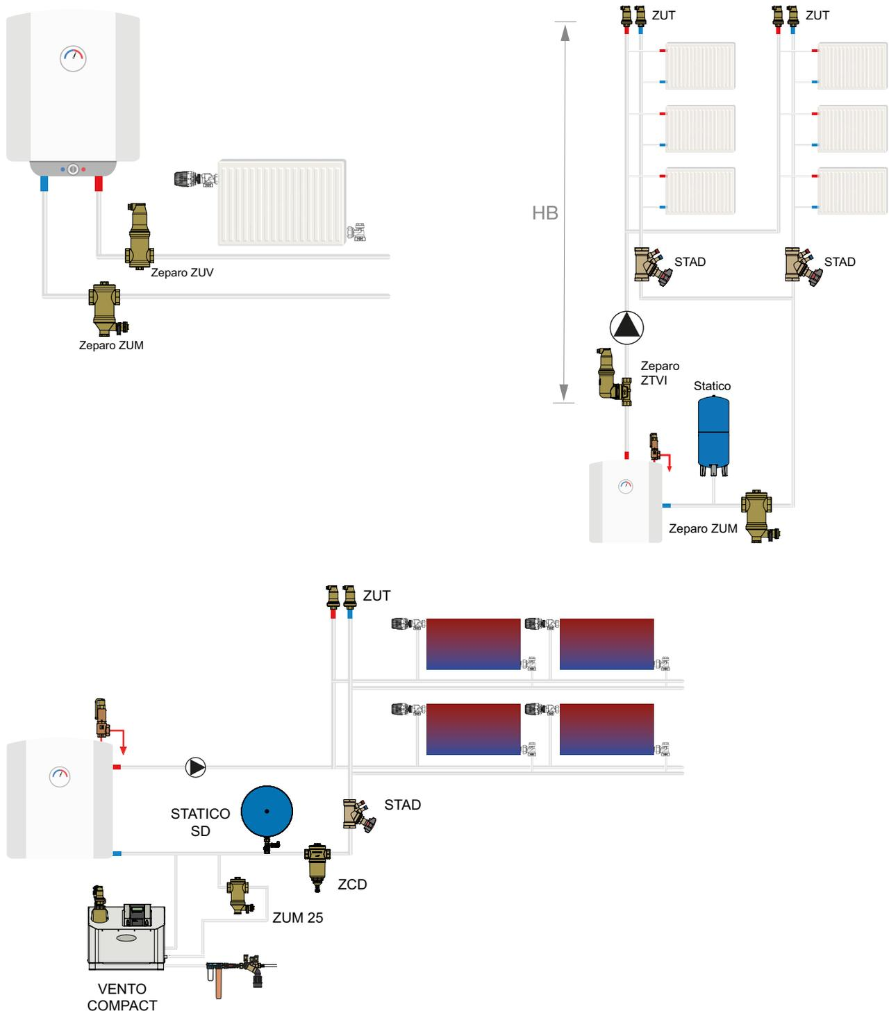
Radiator system with fixed gas cushion expansion vessel
