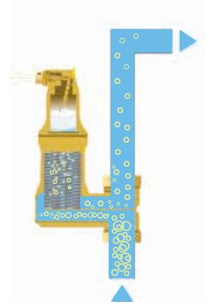
Under normal conditions, microbubble separators cannot achieve undersaturation at the point of installation. However, large parts of the system that are at higher pressures can become absorptive.
