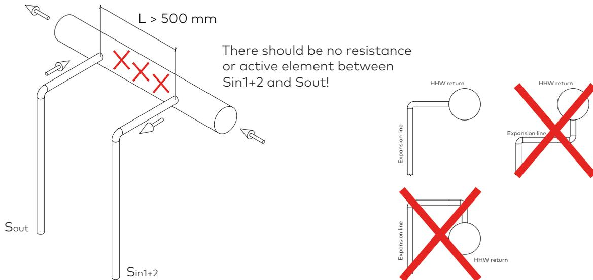
Furthermore, avoid overly long or twisting expansion pipes. Most importantly, avoid vertical loops, which are prone to having air pockets, especially in the case of Transfero TV and Vento V connect. If unavoidable, manual air vents must be installed on top of such parts of the piping.
