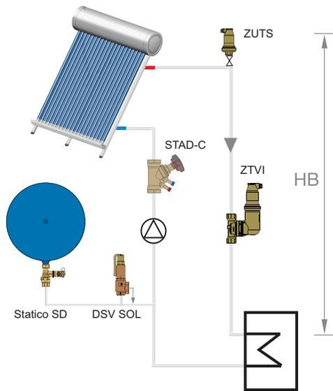
Solar system for higher temperatures and intermediate vessel DD
