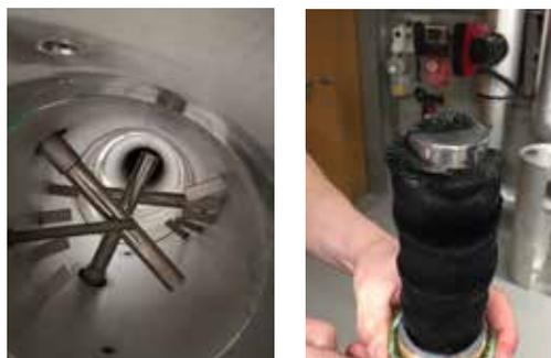
Inner view of a large version Ferro-Cleaner. Example of Ferro-Cleaner efficiency
