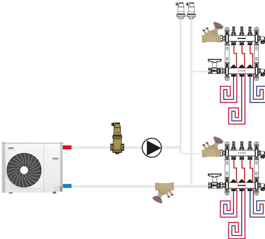
Larger Vento heat pump system with surface heating and vacuum degasser
