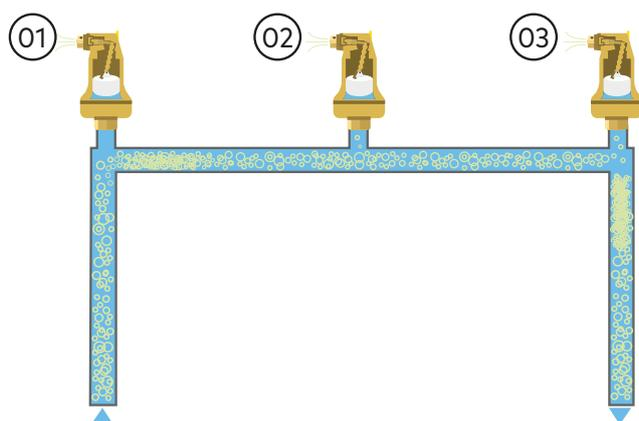
01 This is the worst case, with the bubbles almost completely entrained within the flow.
