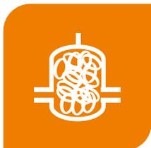
Wire mesh has a combination of turbulent and calm areas. The bubbles collapse in the turbulent area below. Exchange occurs with the calm area above, where the bubbles may then appear.
