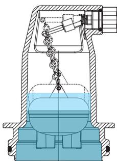
In order to guarantee the permanently perfect functioning of the automatic air vent, it is essential that dirt and water are kept away from the air outlet valve even at high pressures. With Zeparo, this is ensured by maintaining sufficient distance between the water surface and the valve outlet and as well as by the baffle plates below the float, which prevent water from rushing up into the air vent too quickly.
