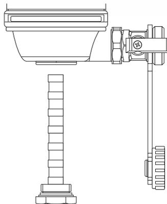
Helistil insert, dirt particles and sludge guided down into the dirt collection chamber
