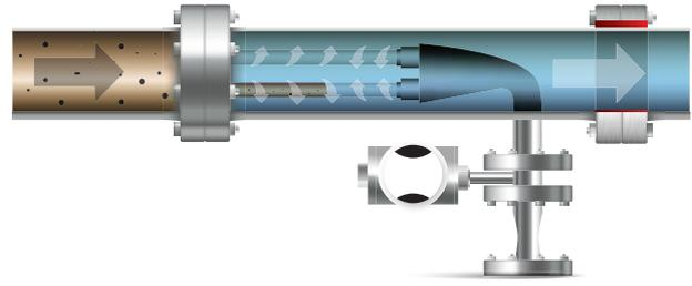
Located at one end of the filter elements is a conical common dirt collector.
