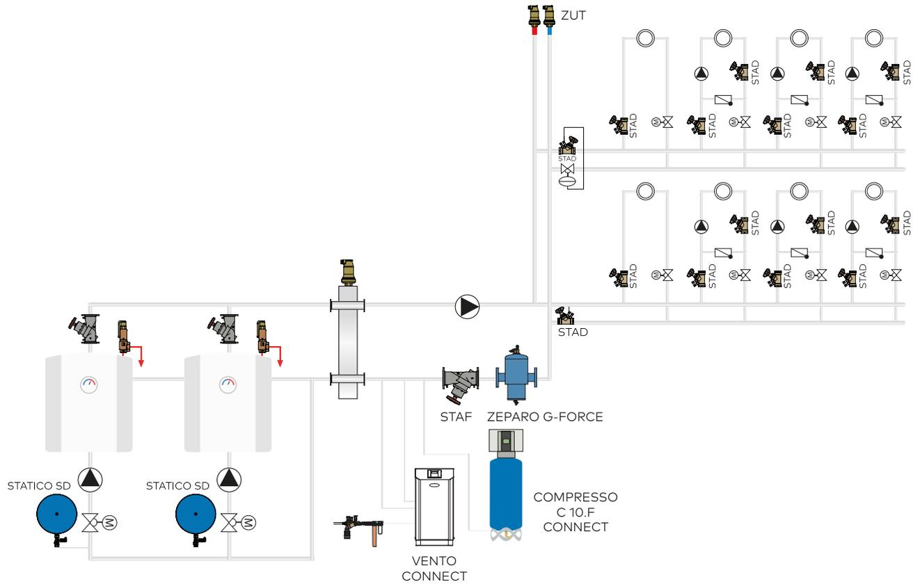
Low loss header with variable flows on the primary and secondary sides
