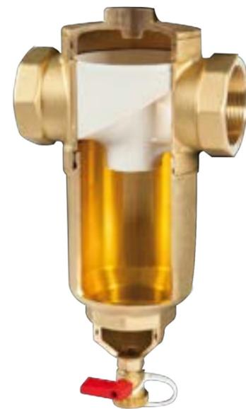
\*For applications where for most of the season, the flow rate is: <20% of qdesign Zeparo ZT turnable is the best choice. >60% of qdesign, Cyclonic technology is the best choice. Between 30%-60% of qdesign, both technologies yield excellent results
