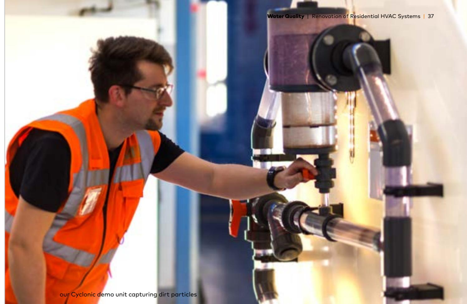
our Cyclonic demo unit capturing dirt particles
